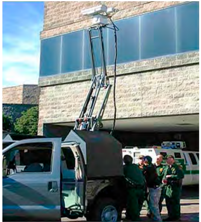
Mobile vehicle surveillance systems provide the flexibility to adapt to dynamic border conditions.
